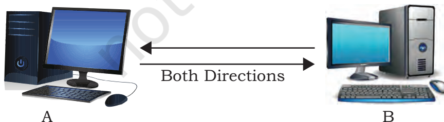
Figure 11.5: Full duplex transmission of data
